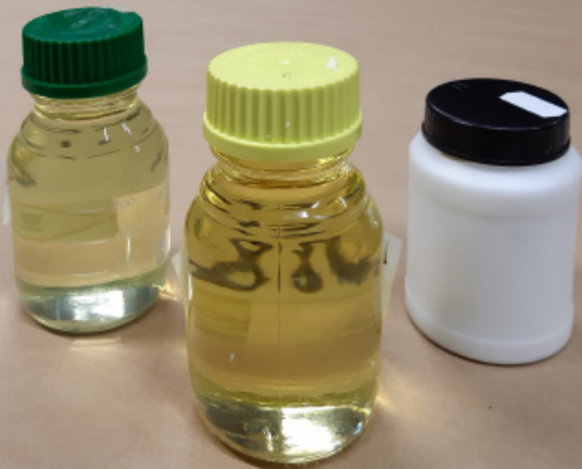
Figure 9. Epoxy resin based on linseed. It consists of: modified epoxy, hardener, flame retardant.
