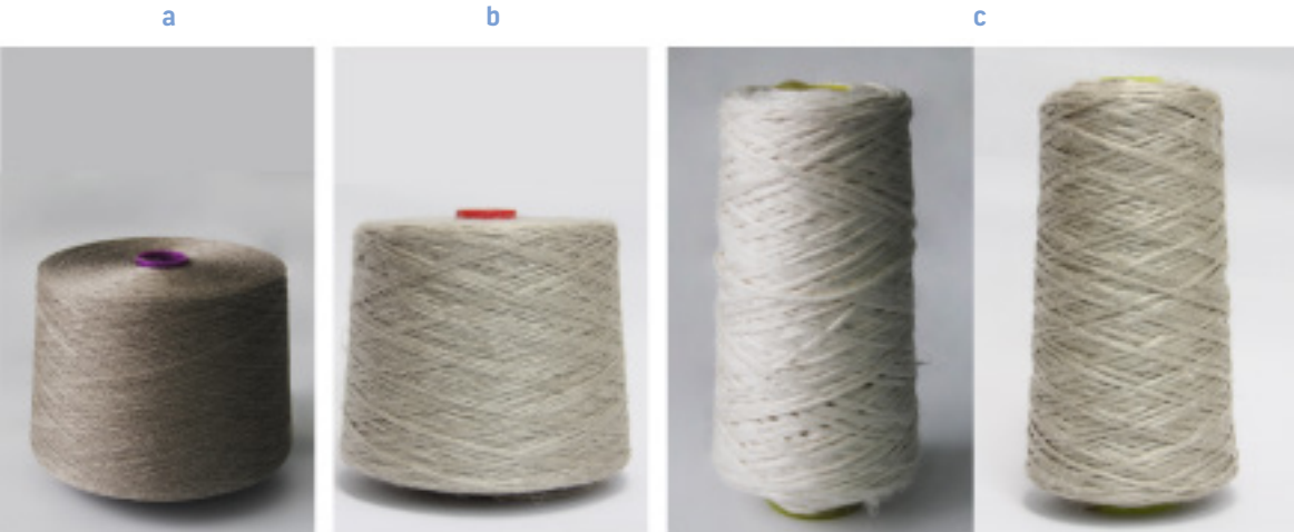
Figure 4. Low-twist yarn of the linear mass of 68 tex (a), rovings of the linear masses of: 400 tex (b) and 2000 tex (c) natural and bleached.
